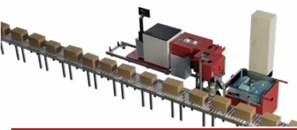
System for the automatic printing, folding and applying of shipping labels and documents
